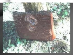
Remakes of pykrete have been made out of newspaper to give a lattice structure like fiberglass – much stronger than original. (Mythbusters, Ep 115, 2009)
