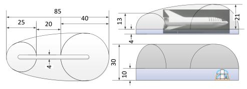
larger structures are 10 meters tall to permit full Starship cargo-scale hardware to fit through airlock doors and passages within the main base. The shorter dome with 4-meter stem walls is for remote installations like spaceport utility housing.
