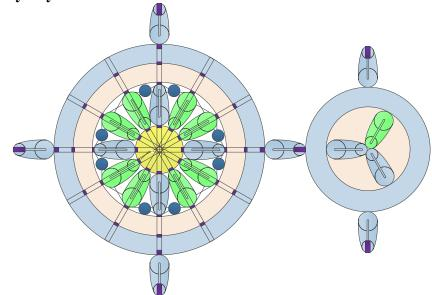
diameter. The dark blue cylinders are storage silos with dome ceilings, 25 meters in diameter. The green domes are agricultural spaces, and the blue ones are airlocks or work areas.
