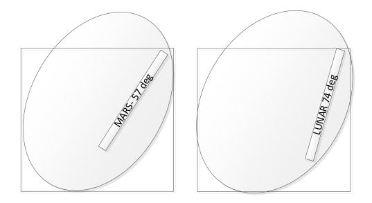
The outer ring has a track that would accommodate a spinning structure for artificial gravity. This is 57 degree slope for Mars gravity or 74 degrees for lunar gravity.
