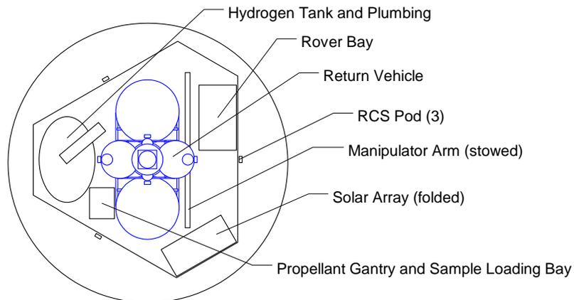
The lander deck contains the hydrogen tank and plumbing, propellant and sample handling gantry, a solar array, a manipulator arm, the rover, and the return vehicle. To better show the return vehicle, the deck equipment has been removed from the side views above.
