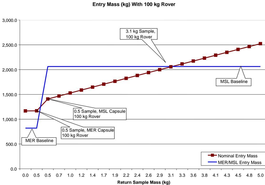
For this illustration, all the rovers are simply scaled up to 100 kg rather than making them proportional to the remainder of the vehicle. Note that the maximum sample size now drops from 3.3 kg (with a 68.7 kg rover) to 3.1 kg. In other words, with the addition of 30.3 kg of rover mass, we only cut 0.2 kg from the sample return mass.
