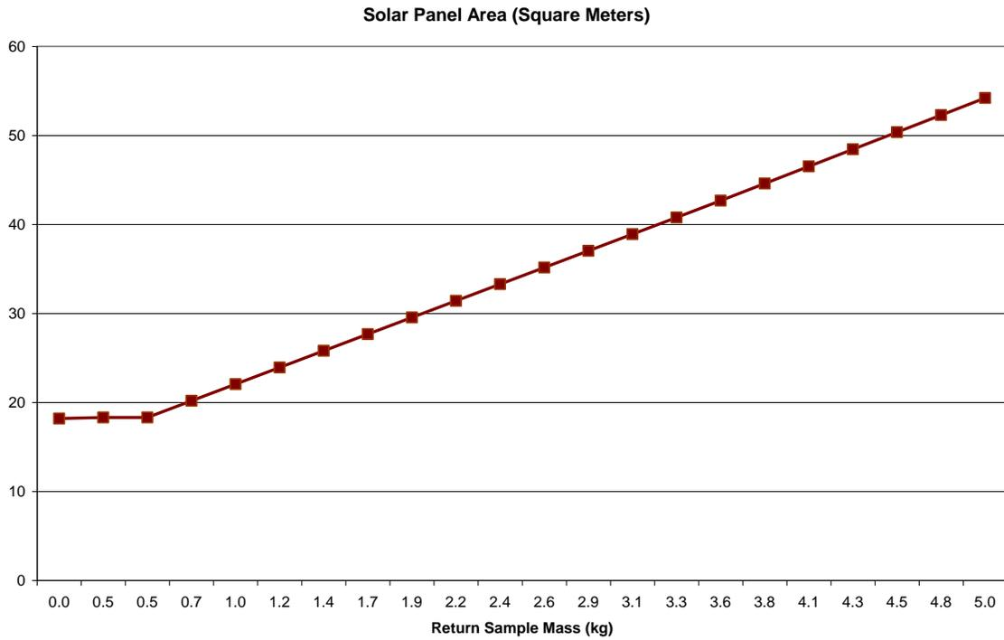
The real problem for scale is shown above. Even an empty sample capsule requires an array of 18 square meters. Cost, ballistics, mass, and other technology issues are less limiting than the issue of how much solar array can deploy autonomously, in rough terrain, with a high likelihood of success, while being packed into the smallest, lightest configuration possible.
