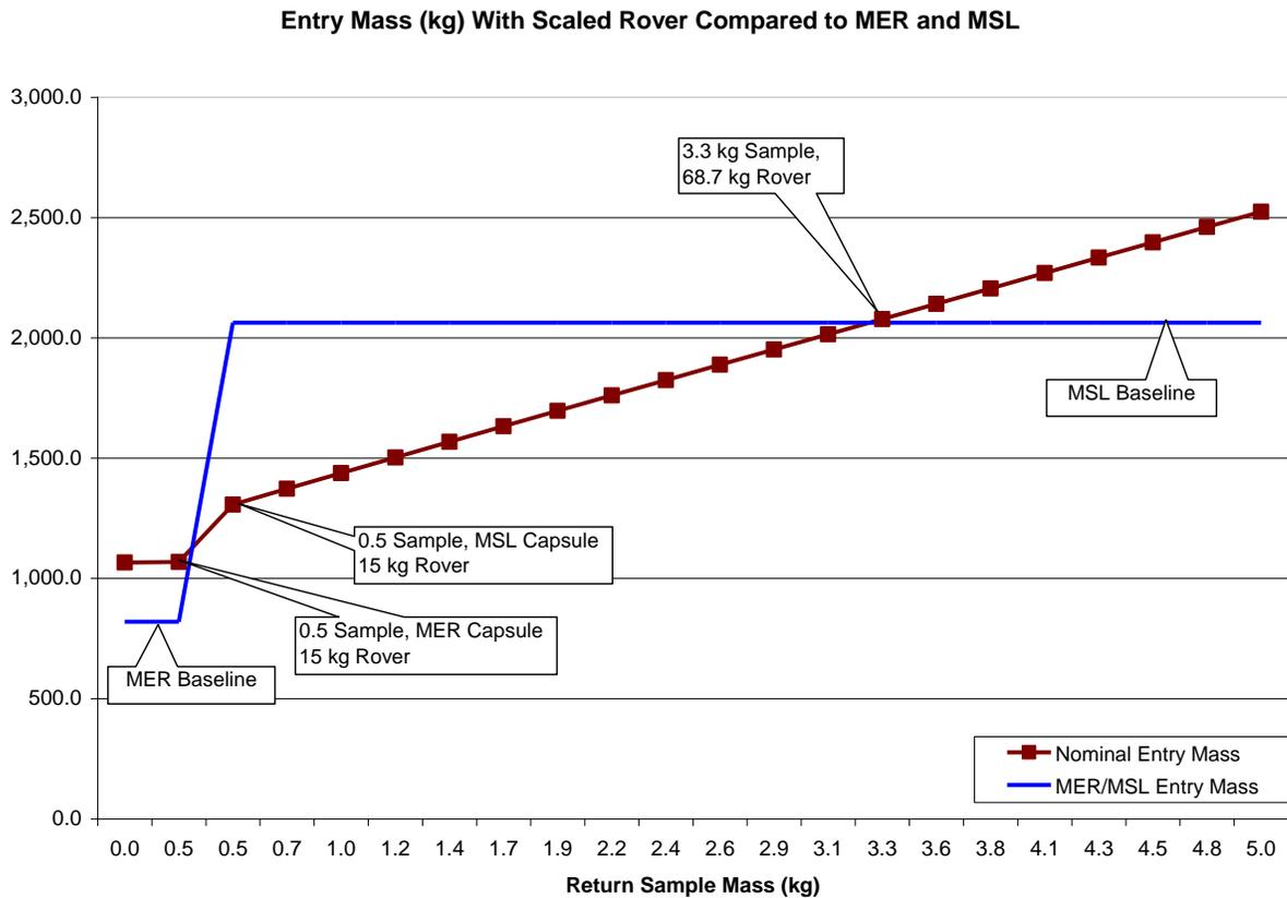
The term “Scaled Rover” means that the rover mass is scaled to the mass of the overall vehicle, with data points evenly spread from 20 kg on the low end to 100 kg on the high end. For reference, Sojourner is 10.6 kg [5] and the MER rovers are 174 kg [7]. It is assumed that even without a rover, local sampling equipment for drilling would still be roughly 20 kg.
