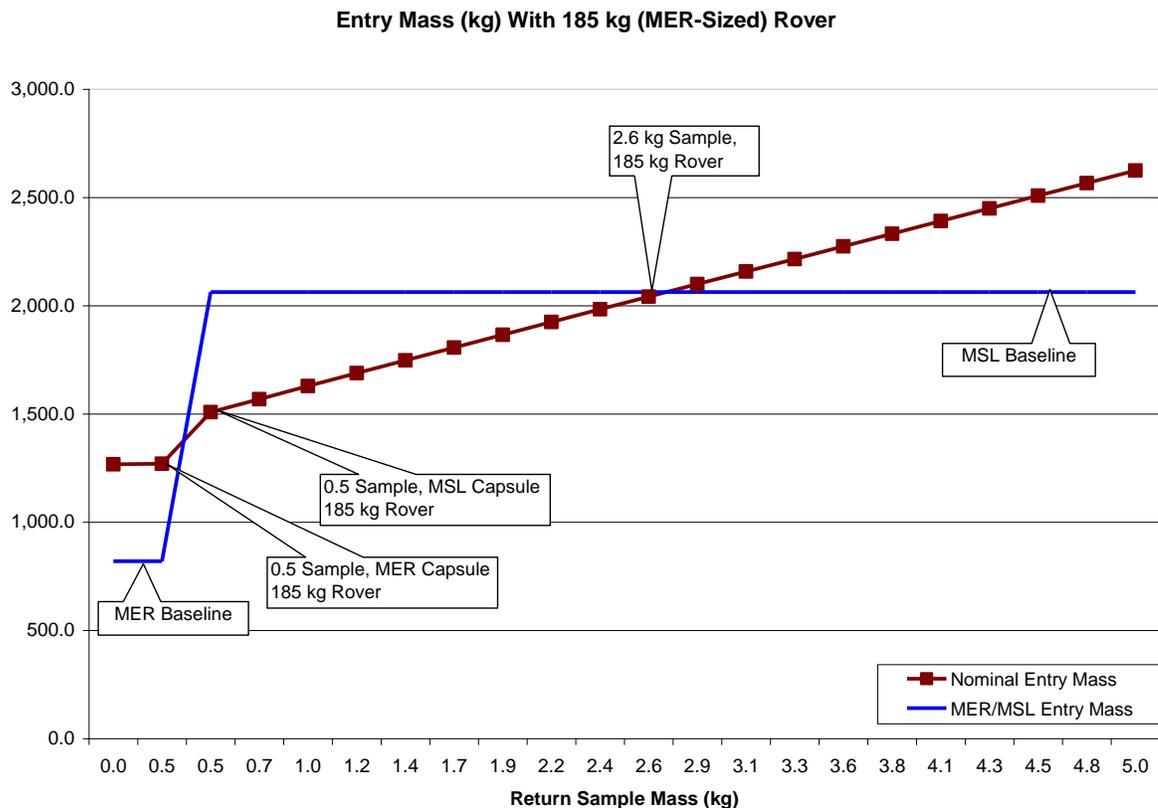
Increasing the rover to MER proportions has dropped the maximum sample size to 2.6 kg – which would still require 35.16 square meters of solar array to power the In Situ Propellant Production (ISPP) system. If the sample is scaled down to 0.5 kg, and the rover remains the mass of the MER, we still have a vehicle that is 73.1 percent the entry mass and 77.5 percent the launch mass of MSL. This is the initial, idealized iteration. However, these are very broad margins to work with.
