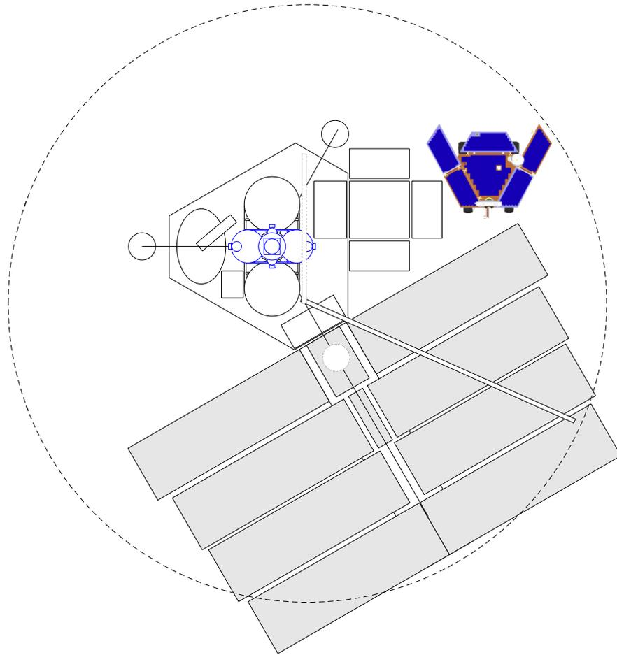
The manipulator arm has sufficient sweep to clean the vast majority of the array directly (dashed circle). While the rover is parked on either side of the array, it too can be cleaned without dependence on dust devils. See also Lander: Manipulator Arm.
