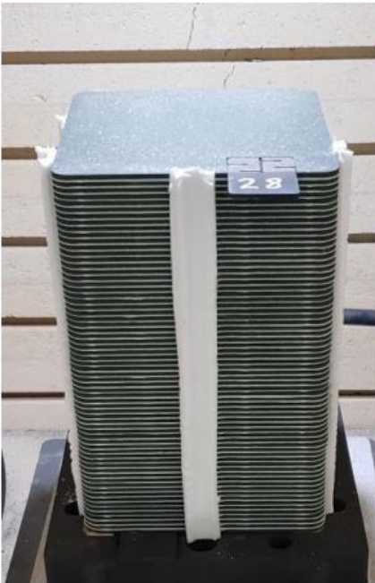
Figure 5. ISRU design variant 65-Cell SOXE, internally manifolded with sealed perimeter.
