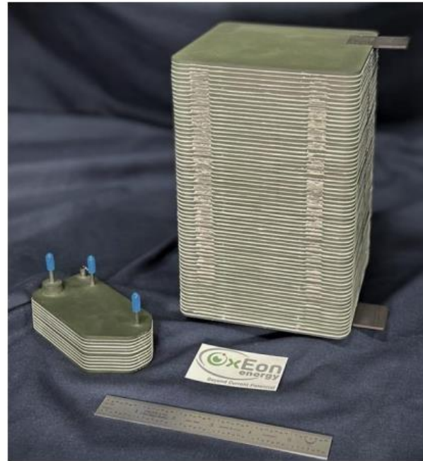
Figure 6. Size comparison of SOXE stacks from MOXIE and NextSTEP projects.
